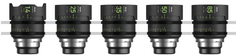
All NiSi Athena Prime lenses are matched in weight and size, which means they do not require rebalancing on a gimbal when switching between lenses. The 77mm filter thread and matched aperture and focus rings across the range also make it easy to use lens accessories such as filters and focus gears. The focus ring features 300° of rotation with fluorescent focal scales for precise focus pulls.
